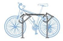
6. Dual height racks need assisted lift. A gas strut is a good example of how to achieve this.
