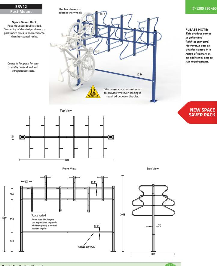
Material Specifications (General) 70 x 70 x 2.5mm Post / 34 x 3mm Beam / 60 x 30 x 2mm Angle 19 OD x 1.2mm Rail / Hot dipped galvanised
