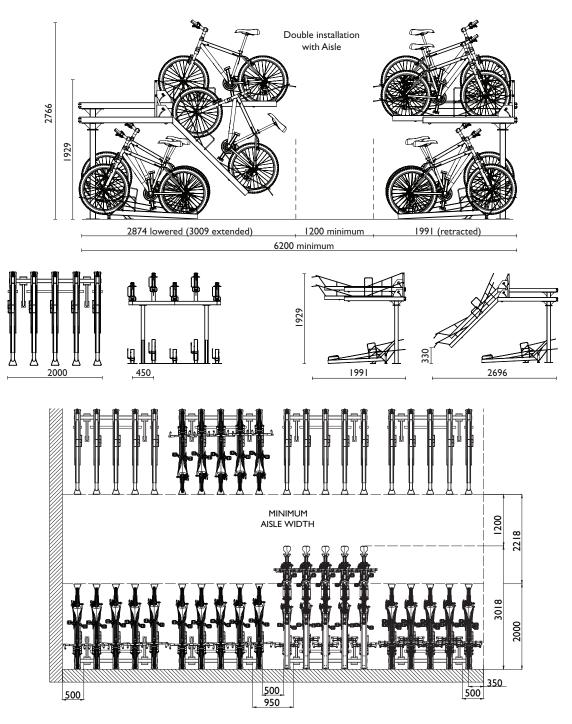
Material Specifications (General)Frame80 x 80 x 3mm SHSFinishHot dipped galvanised
