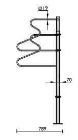
Material Specifications (General) 70 x 70 x 2.5mm Post / 34 x 3mm Beam / 60 x 30 x 2mm Angle 19 OD x 1.2mm Rail / Hot dipped galvanised
